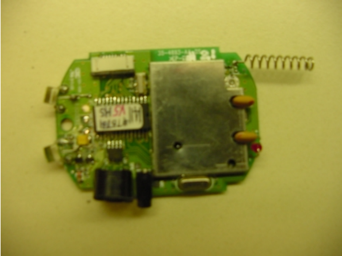
Front of Circuit Board for Handset
