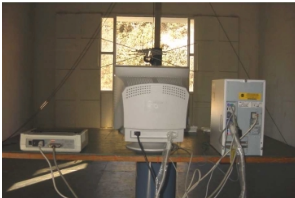
Figure 2(a) : Radiated Emission 30MHz ~ 1000MHz
