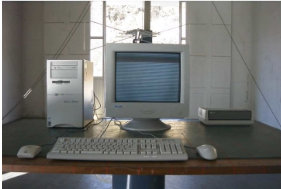
Figure 2(a) : Radiated Emission 30MHz ~ 1000MHz
