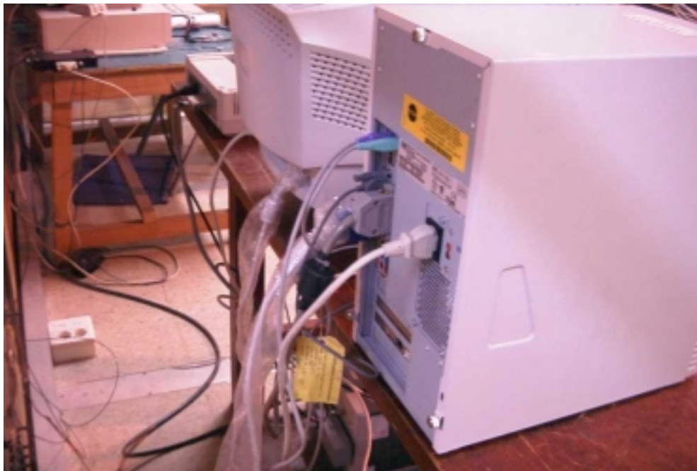
Figure 1(a) : Conducted emission 450kHz ~ 30MHz
