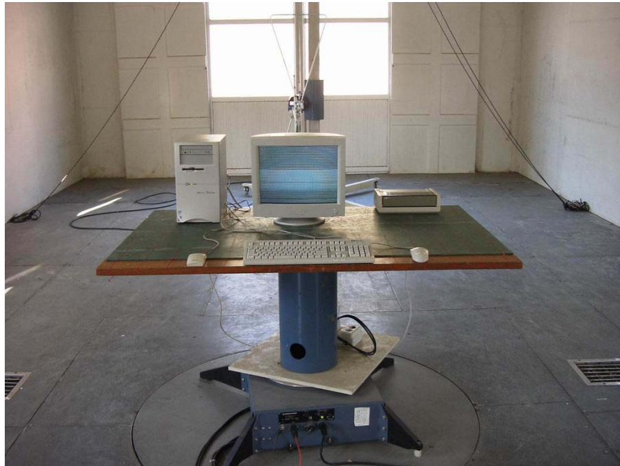
Radiated Emissions 30 MHz - 1000 MHz
