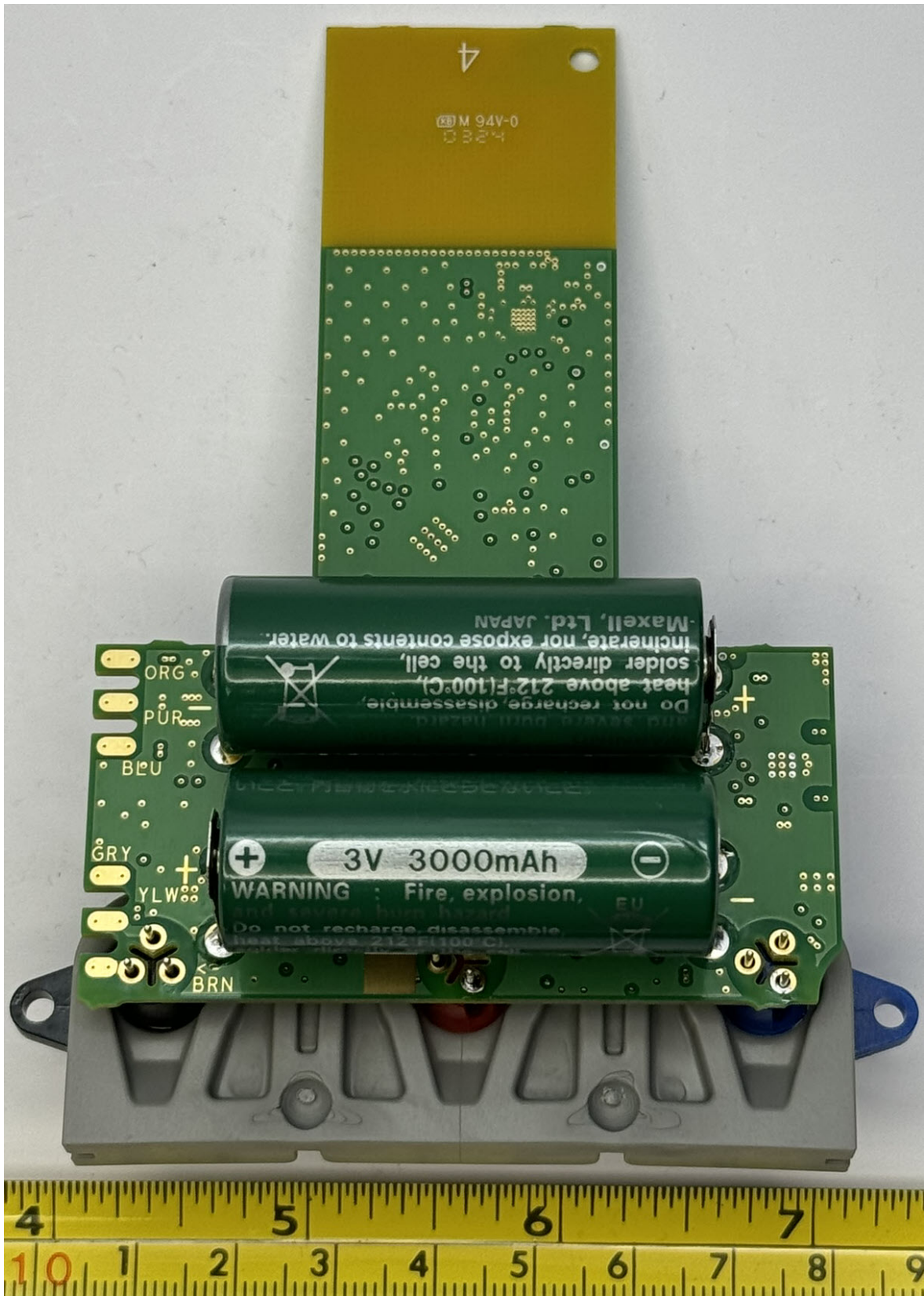
Figure 2.9: Pit 2-Battery, 3-Port - Back
