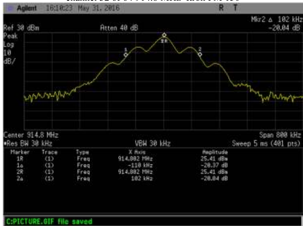
channel 32 of 64 914.8 MHz Itron FM 150
