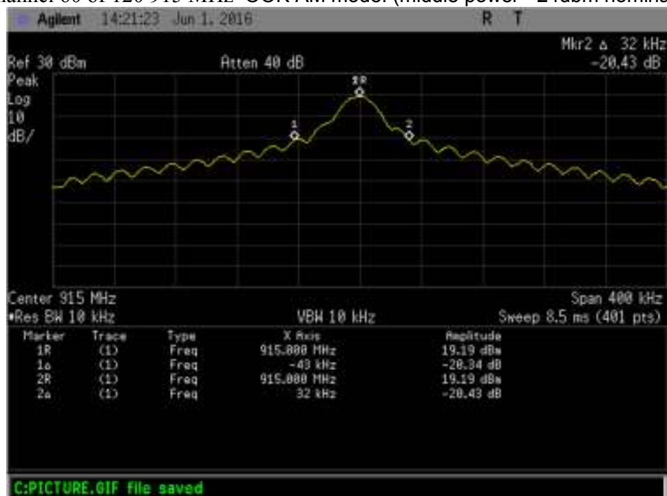
channel 60 of 120 915 MHz OOK AM mode. (middle power +24dbm nominal )
