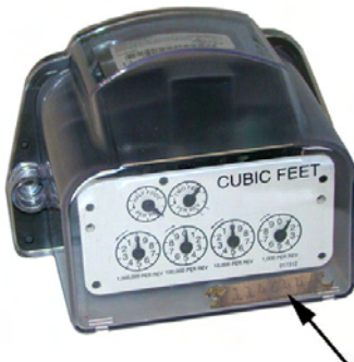
Method 3: Place the brass meter tag inside the ERT module assembly
