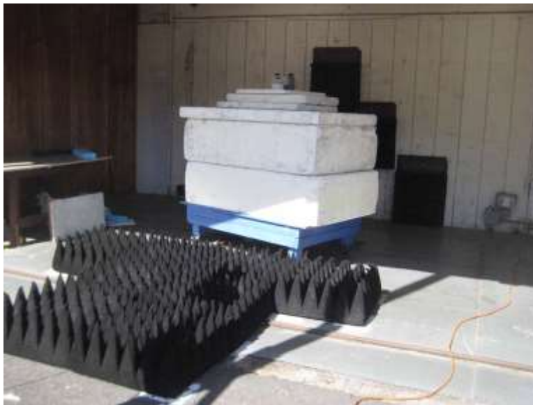
Above 1GHz Cone placement
