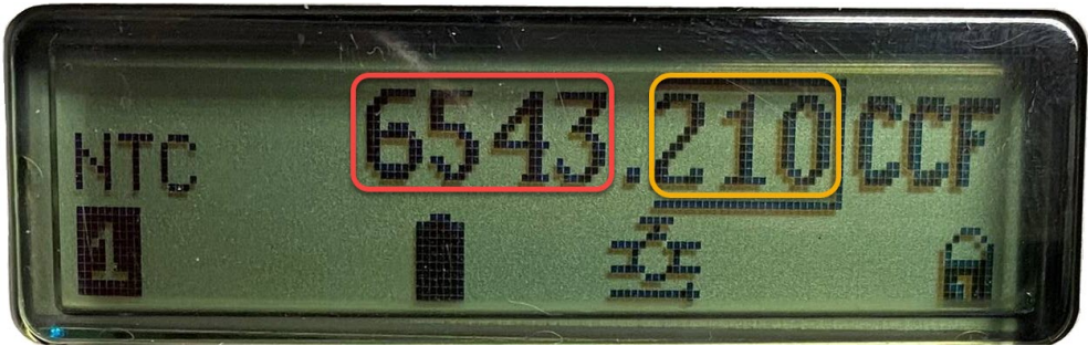
Figure 2 Intelis Gas Meter configurable display
