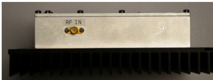
Power Amplifier 3-23365 rear view.
