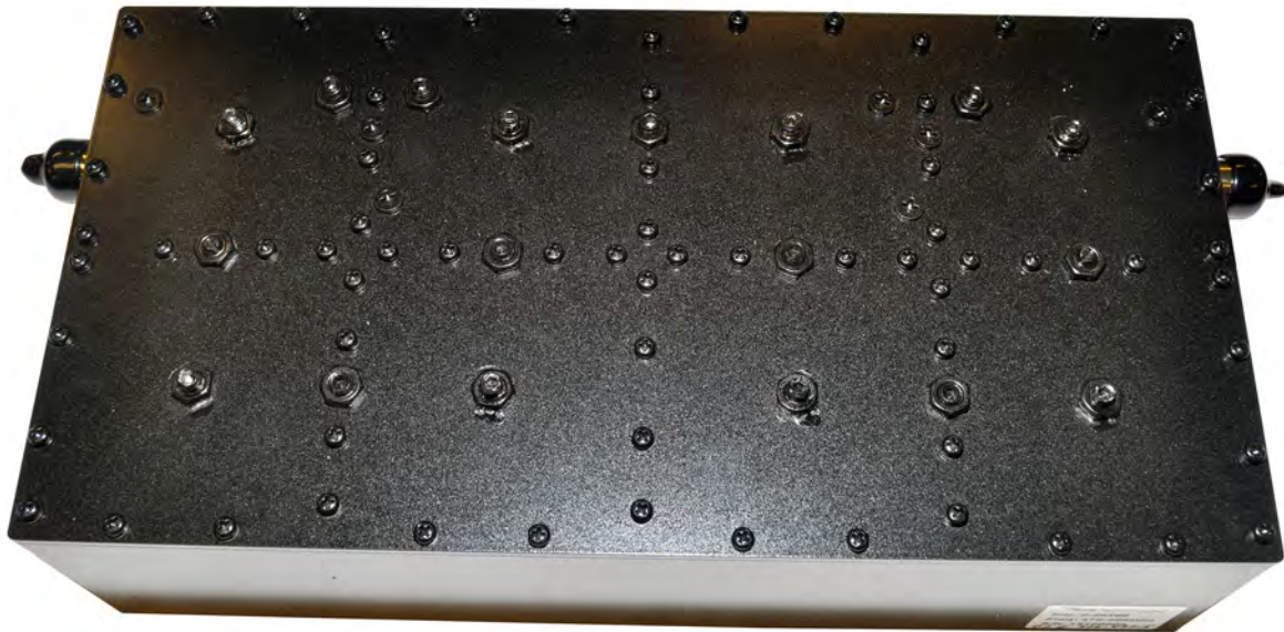
Filter Assembly top view (part # 8-25295)
