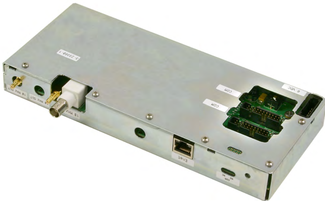
Control Board 3-23360-1 front-right view.
