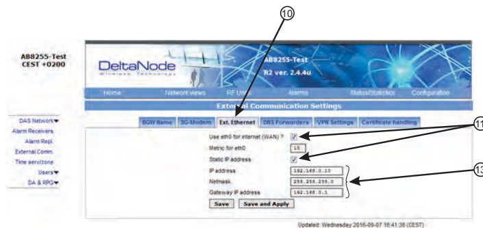
Figure 128 BGW Configuration - External Ethernet Setting
