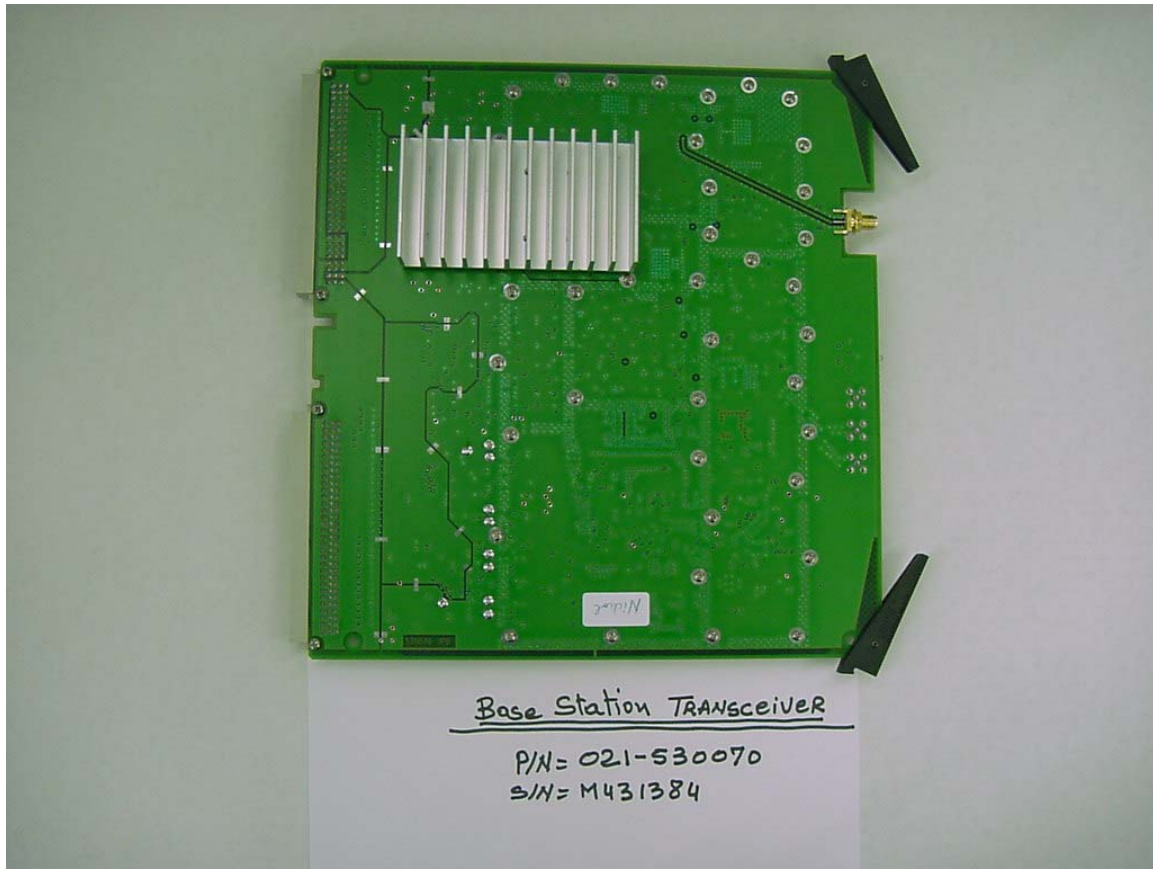
Base Station Transceiver Bottom
