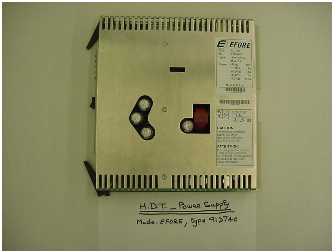
DC-DC Power Supply Top
