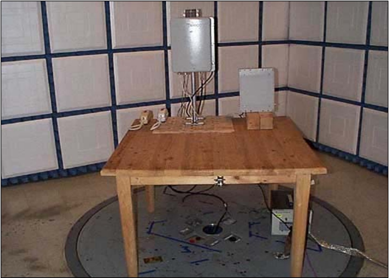
Mains Conducted Emissions - Front View
