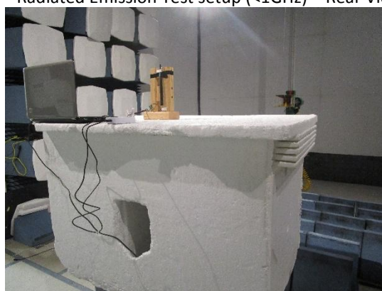
Radiated Emission Test setup (>1GHz) – Rear View
