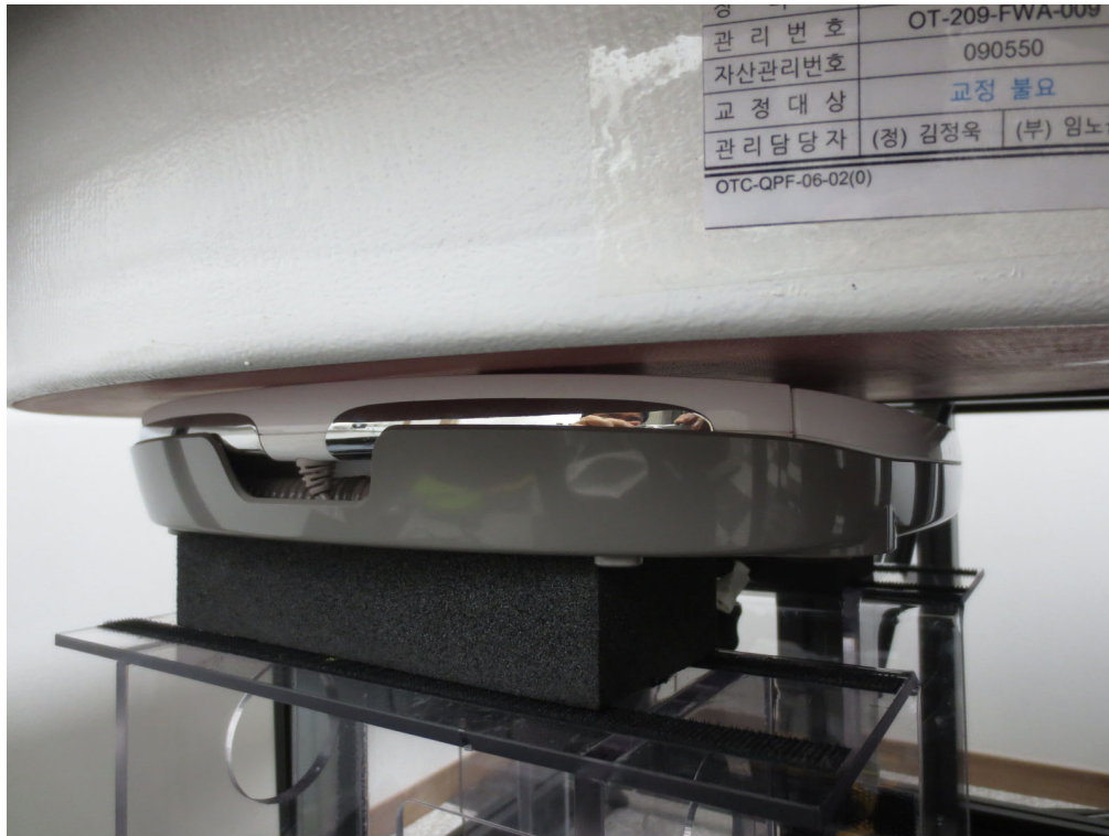
Front from Flat Phantom (Separation Distance: 0 cm)
