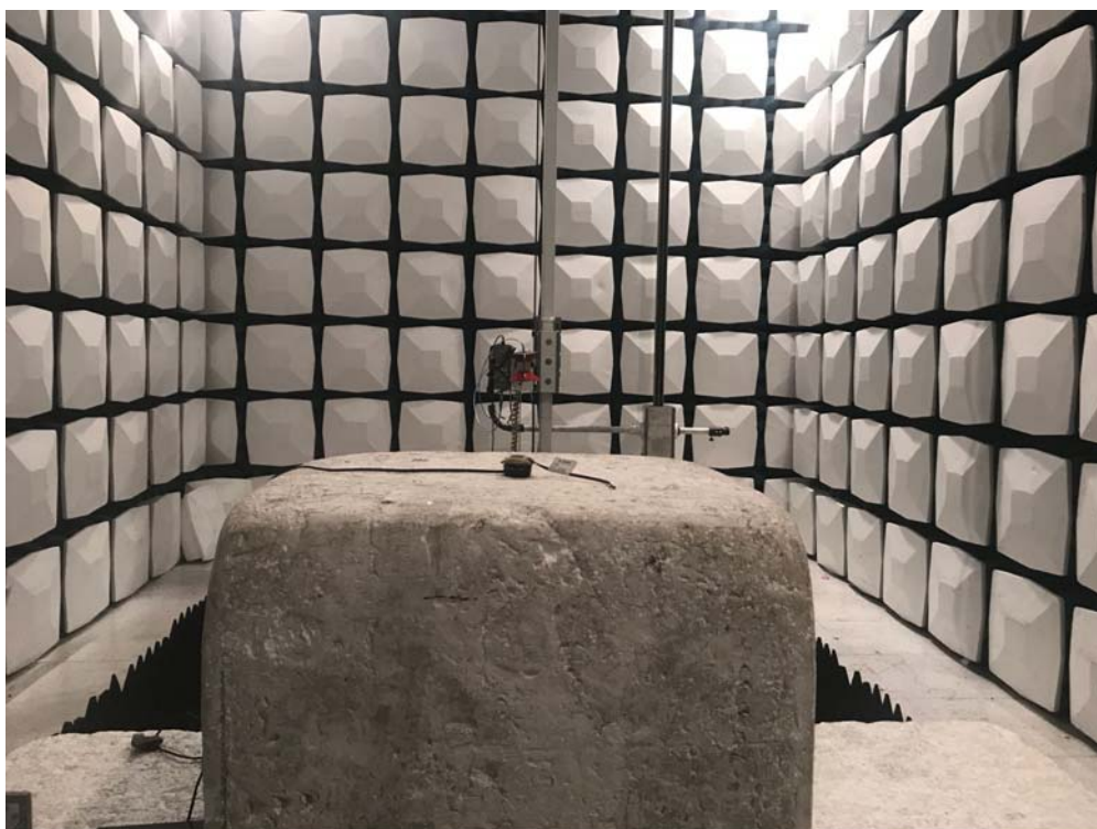
Description: Radiated Emission Test Setup for 1~18GHz
