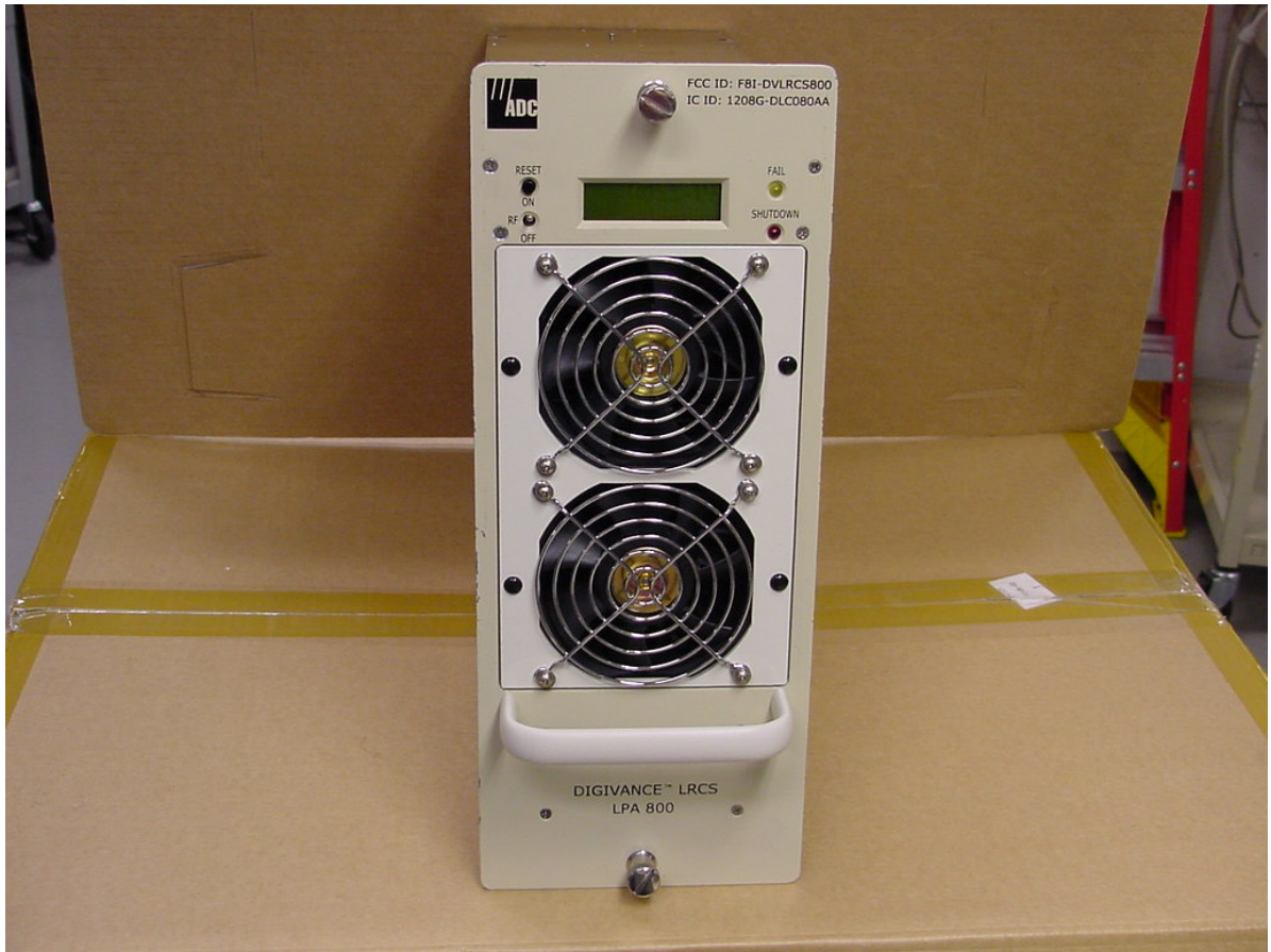
800 MHz Linear Power Amplifier Front View
