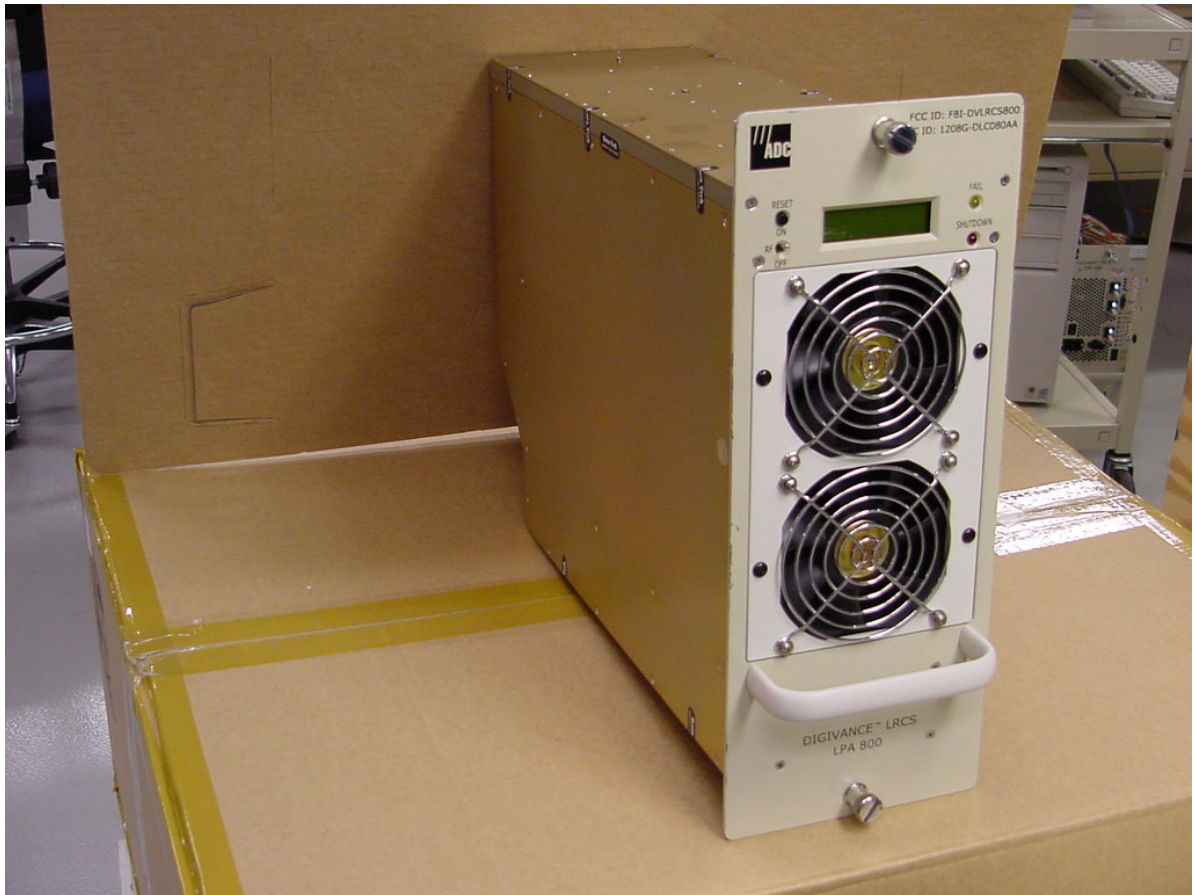
800 MHz Linear Power Amplifier Left View
