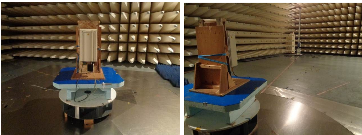
picture 8.2: Test setup: Field Strength Emission <1 GHz @10m in the SAC
