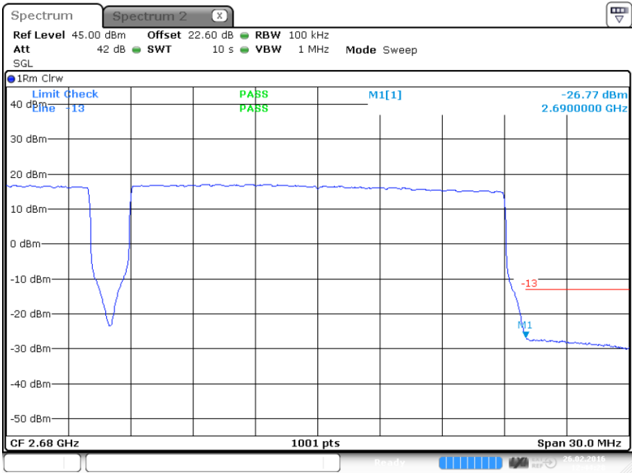
plot 8.3.1.1-#2 Intermodulation: §27.53, §2.1051; Test results; Downlink; LTE Upper Band Edge
