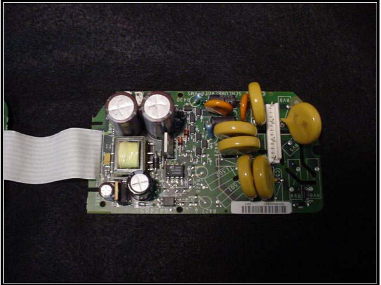
Figure B7: Topside of Power Supply Board
