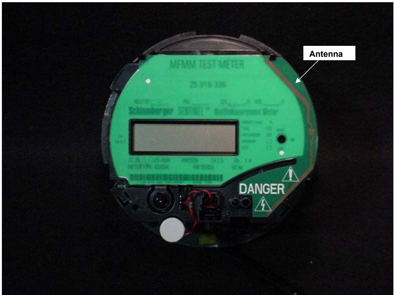
Figure C1: Outer Cover Removed Exposing Face Plate with Antenna
