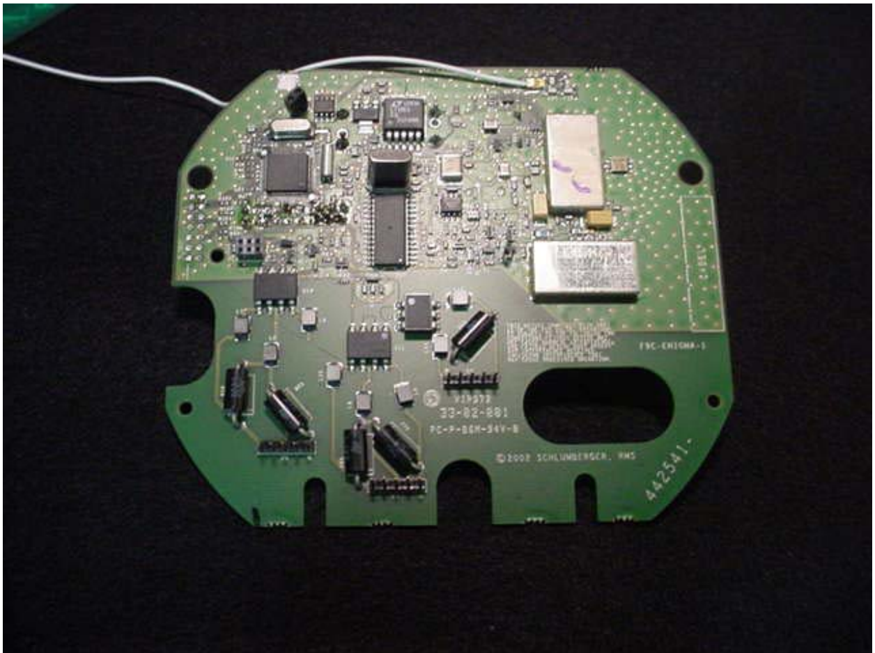
Figure B5: Top Side of RF Board
