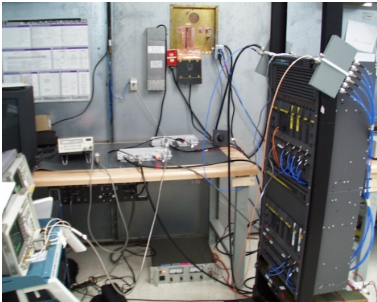
Conducted Spurious Setup at KTL Ottawa Laboratories
