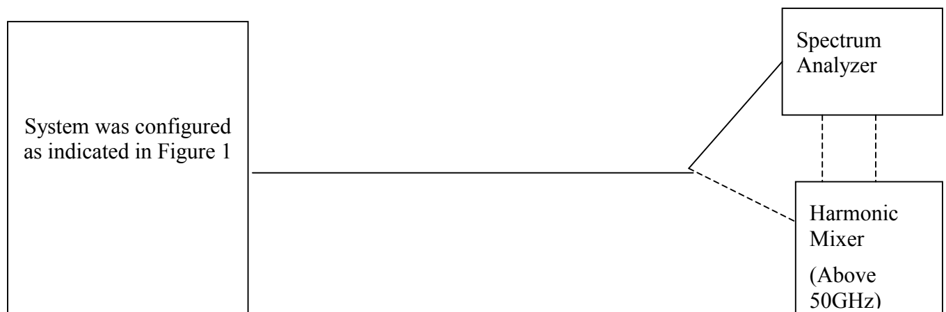
Figure – 5 Conducted Spurious measurement setup
