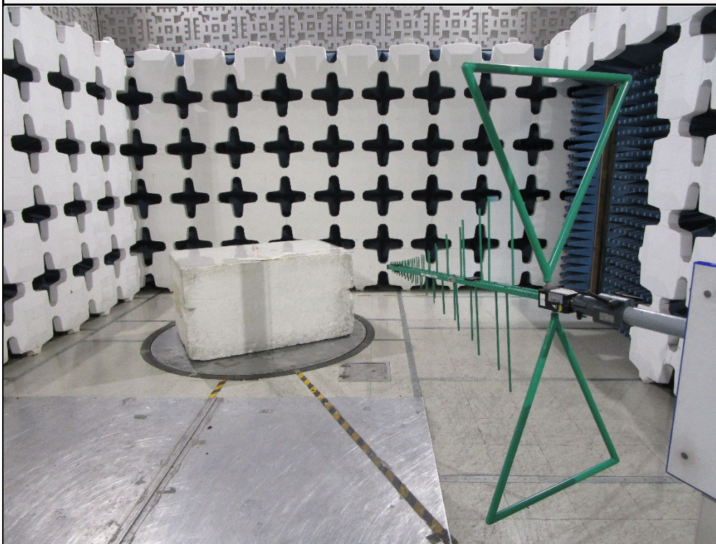
Test Setup for Spurious Radiated Emissions, 30-1000MHz – Antenna Polarization Vertical
