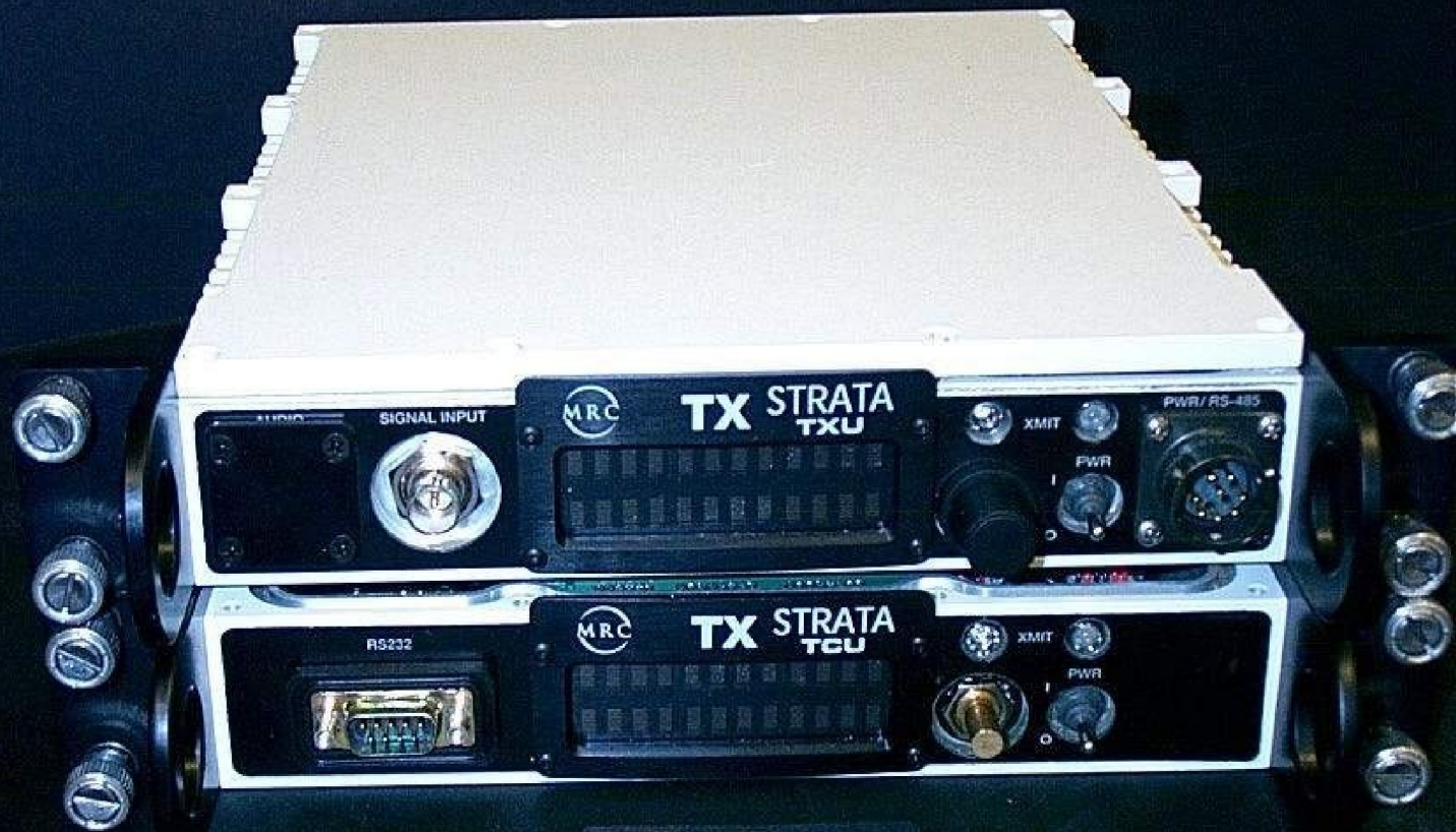
TRANSMITTER UNIT TRANSMITTER CONTROL UNIT
