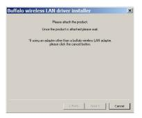
Click *Next* to step through the installation wizards. When the wizard asks you to insert your device, plug the AirStation WLI-UC-GN in to a USB port on your computer. Drivers will install automatically, and if you checked its box, Client Manager 3 will install as well. When the wizard is complete, click *Finish*.
