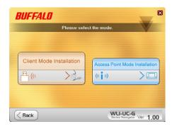
Besides its wireless client capability, the WLI-UC-GN can function as a wireless access point. If your computer already has a connection to the internet, and you want to connect AOSS-compatable devices wirelessly, then choose *Access Point Mode* during installation. Note: If you have firewall or antivirus software running on the computer, temporarily disable it before continuing.
