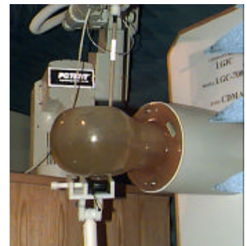
Figure 1. SAR Test Set-up
