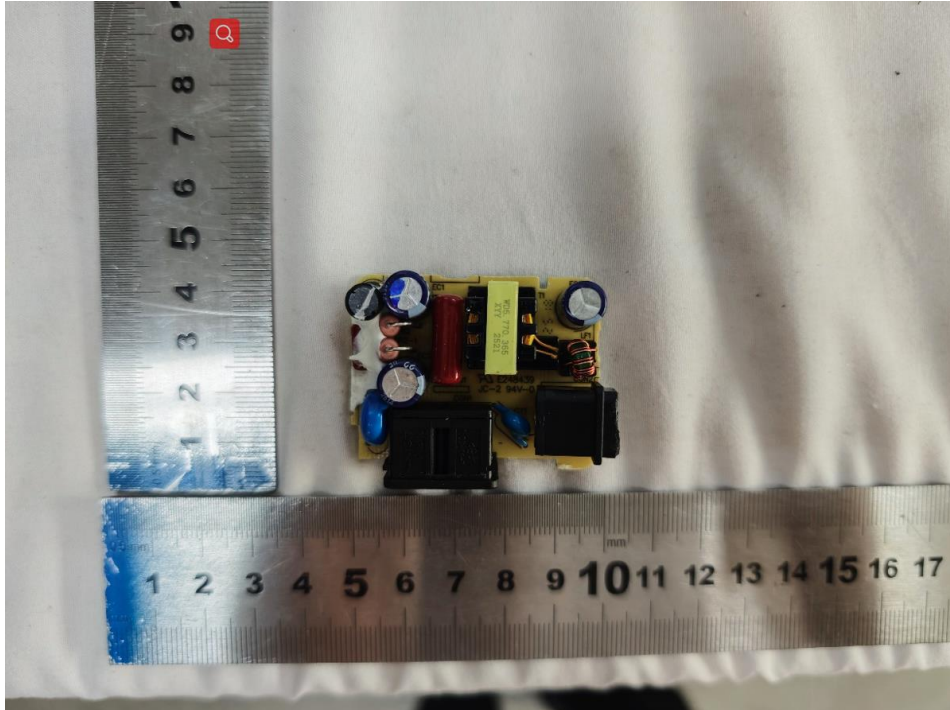
PCB of power supply
