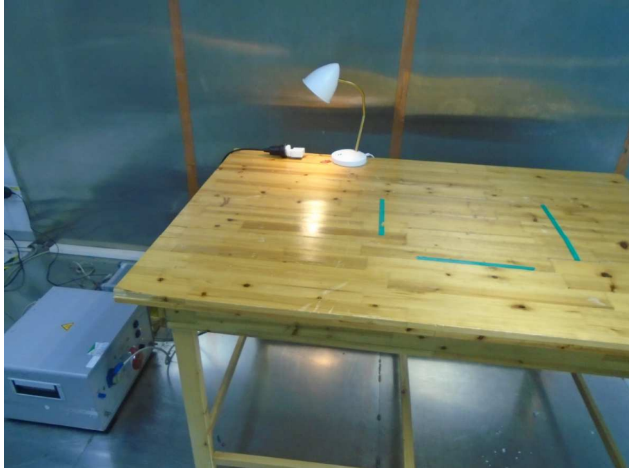
Photograph 1: Set-up for measurement of conducted emission
