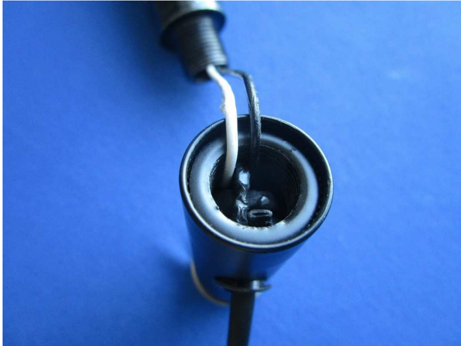
Internal wire with cable anchorage
