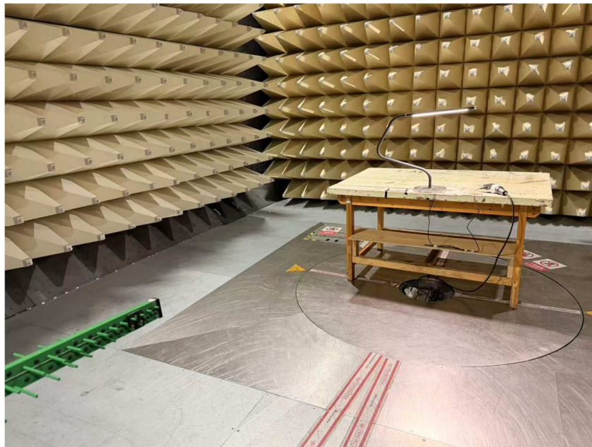
Photograph 2: Set-up for measurement of radiated emission
