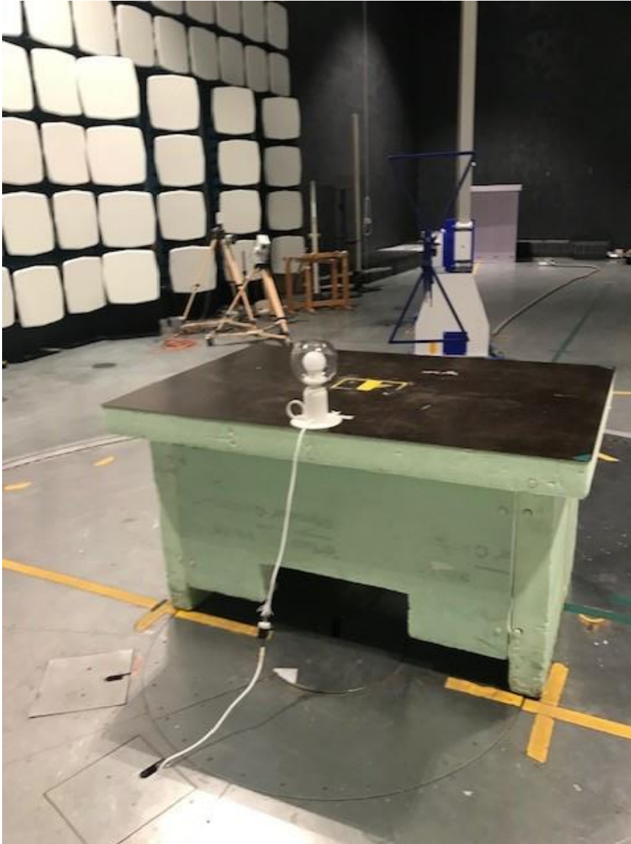
Test set up radiated emission 30 MHz – 1 GHz
