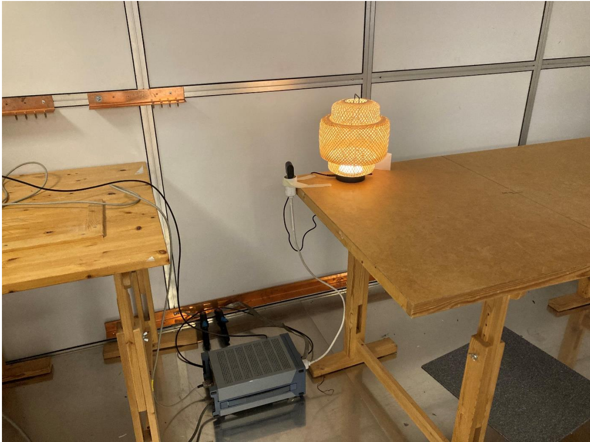
Test setup for conducted emission 150 kHz – 30 MHz
