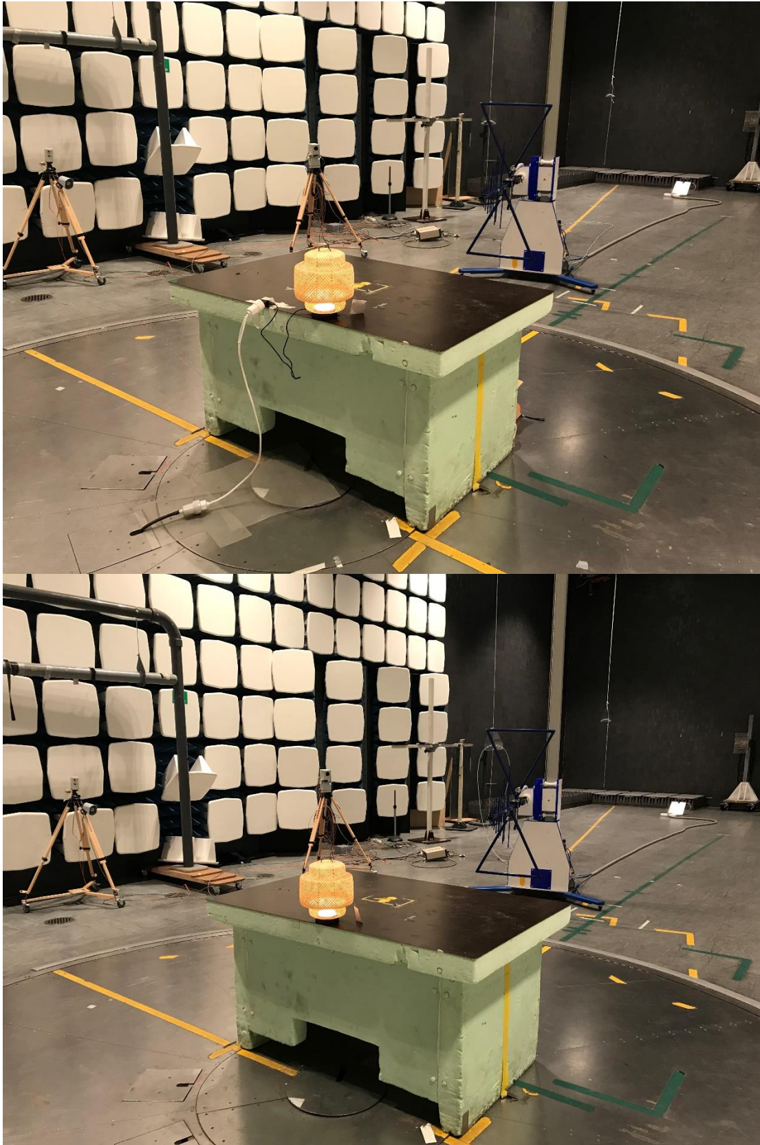
Test set up radiated emission 30 MHz – 1 GHz
