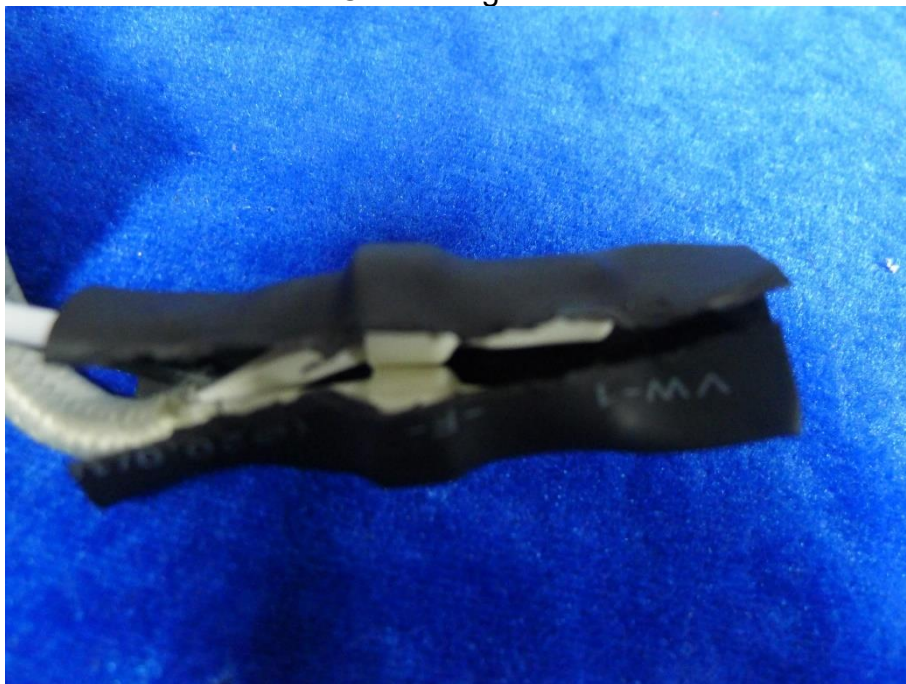
Connecting Point (Heat-shrinkable Sleeve Used)
