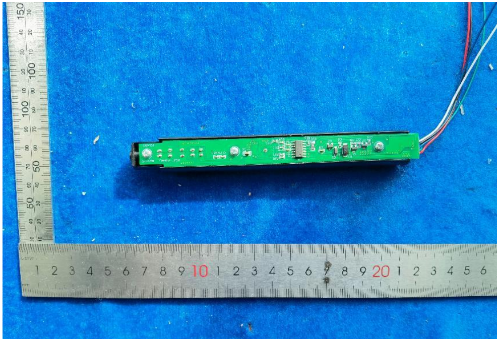
Inside of control module
