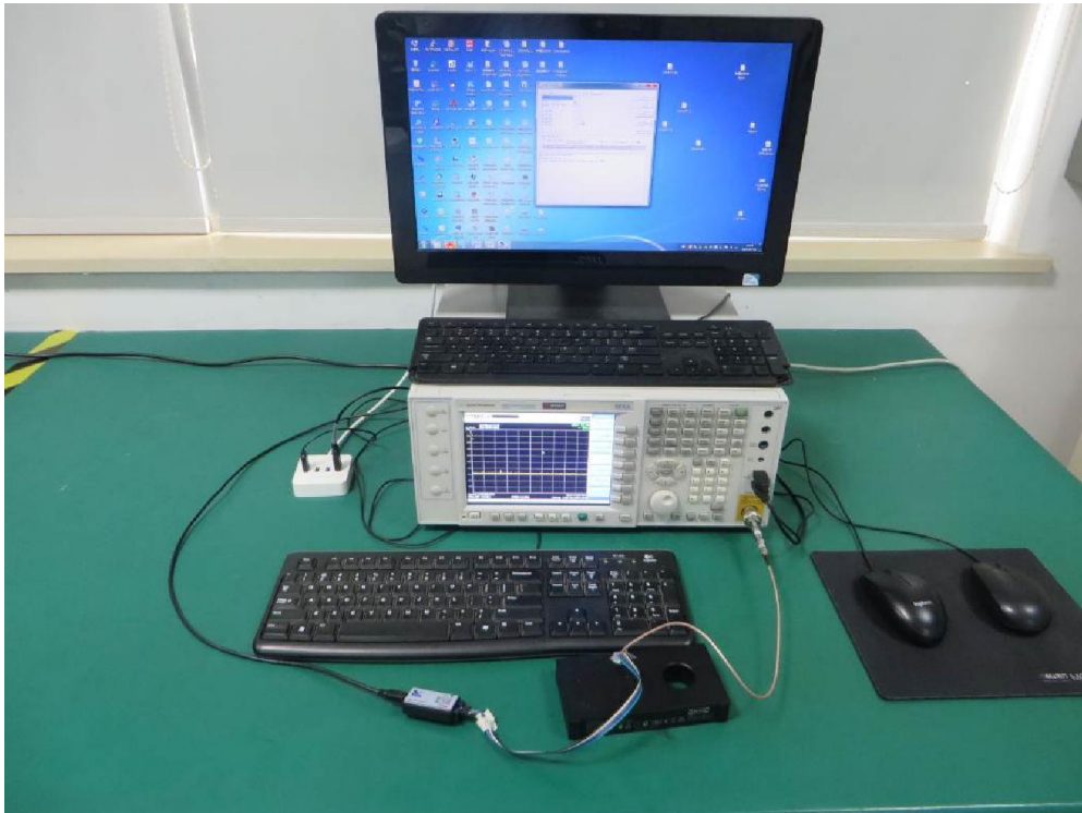
Description: Radiated Spurious Emission Test Setup for 9kHz ~ 30MHz
