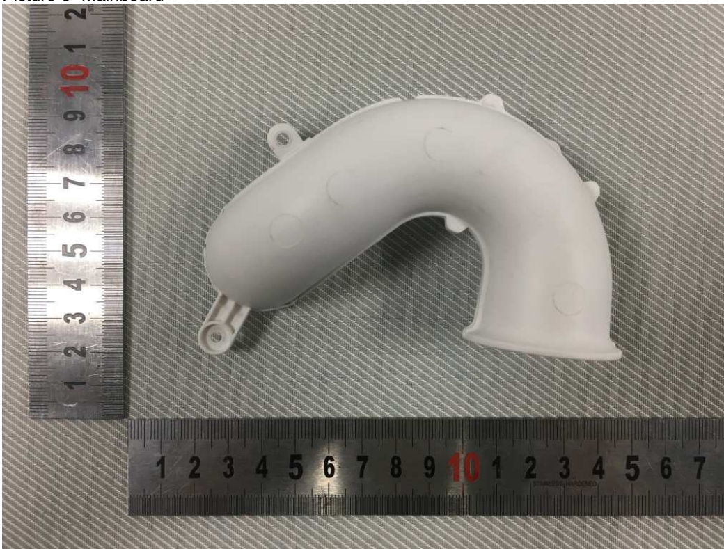
Picture 6- Internal air pipe
