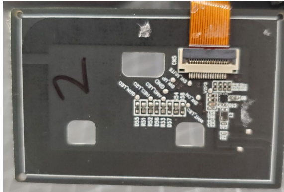
(fig. 7) Back side of LED button NFC board
