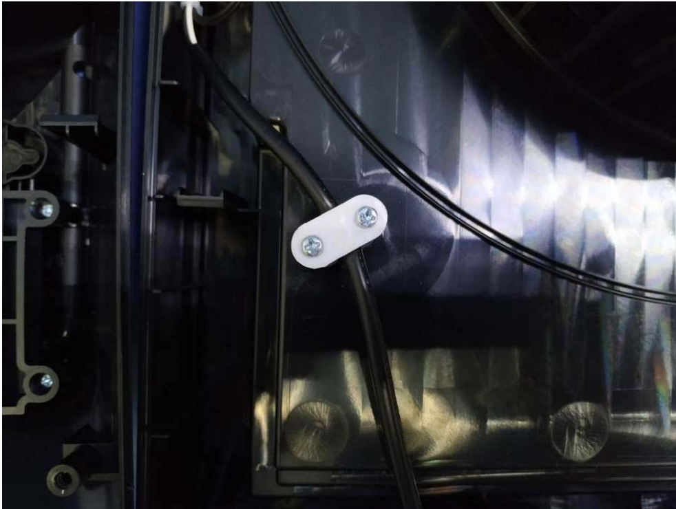
Cord anchorage view
