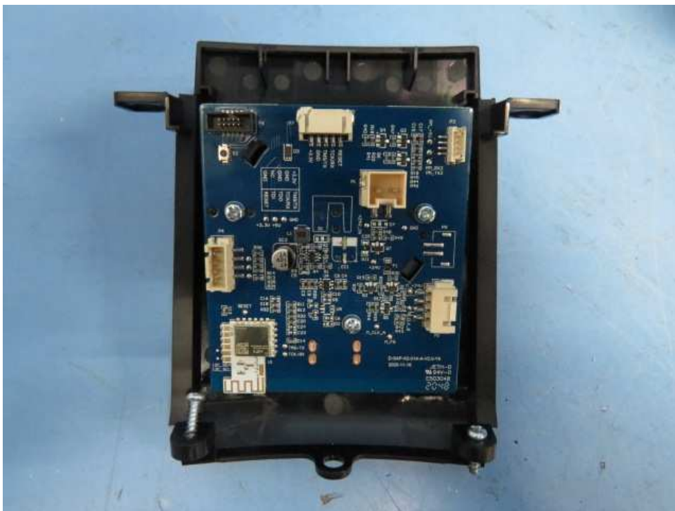
Main control board PCB view
