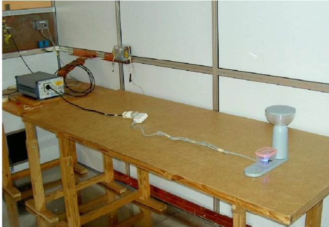
Test setup for conducted emission 150 kHz – 30 MHz
