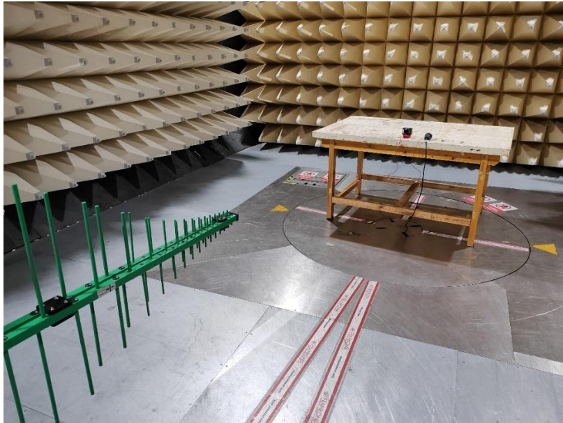
Photograph 3: Set-up for measurement of radiated emission
