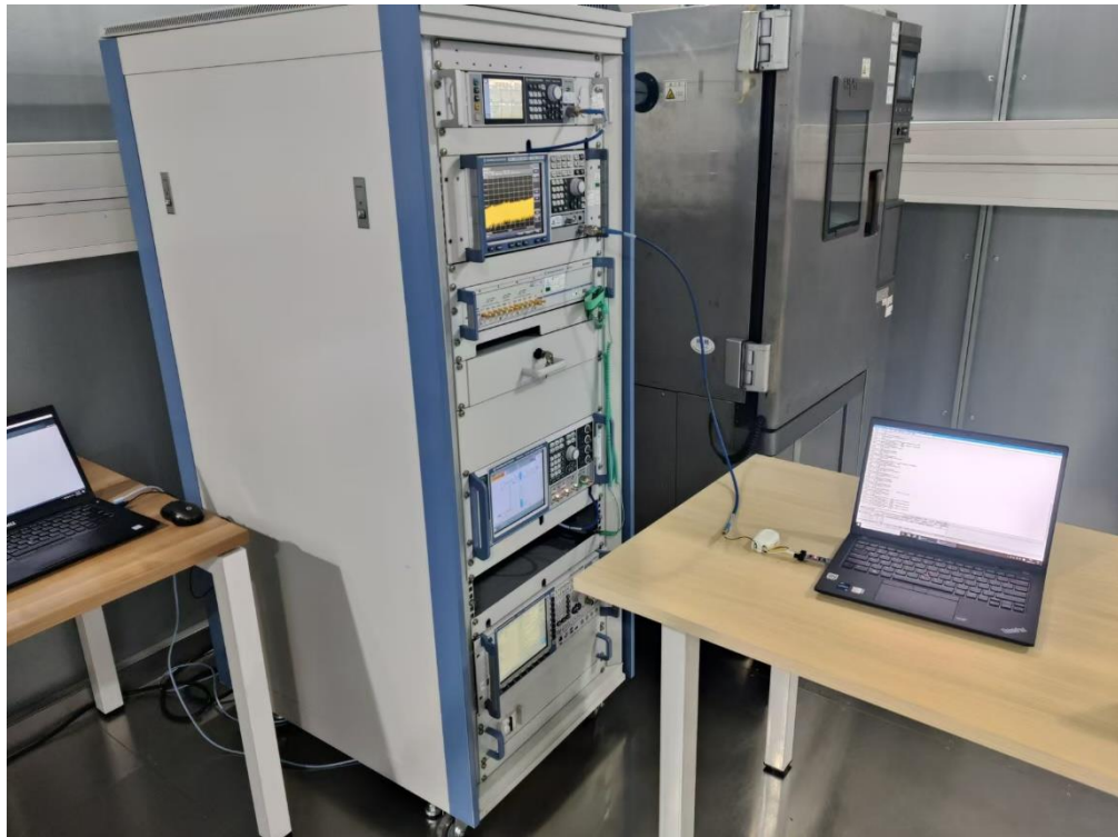
Photograph 1: Set-up photo for RF Conducted Test
