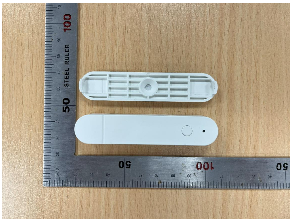
Bild / Picture 2: Overall view with battery lid opened
