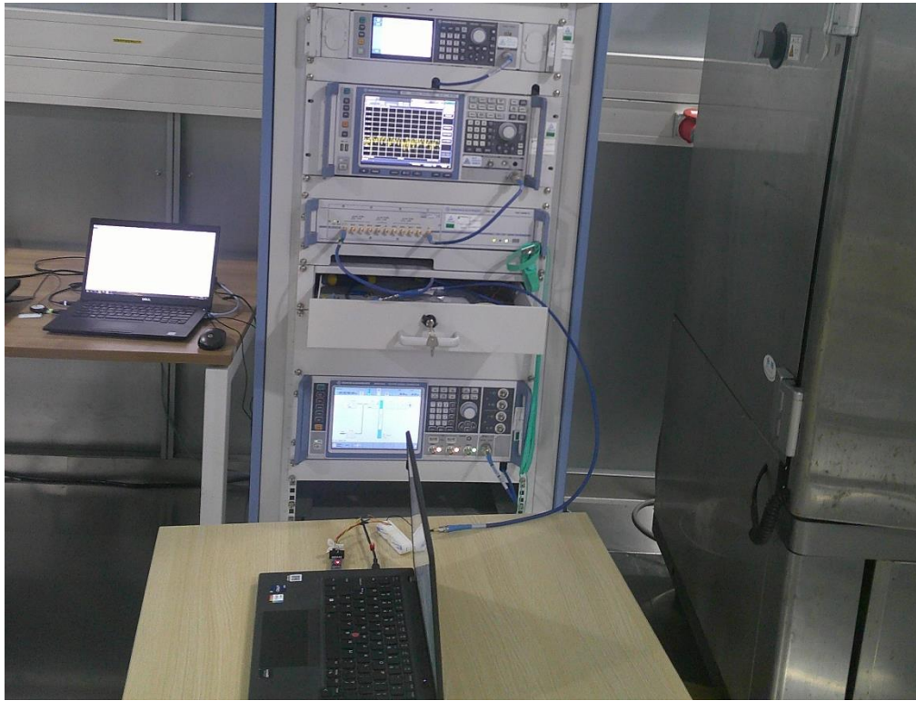
Photograph 1: Set-up photo for RF Conducted Test
