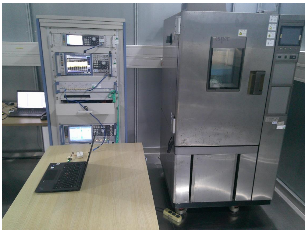
Photograph 1: Set-up photo for RF Conducted Test
