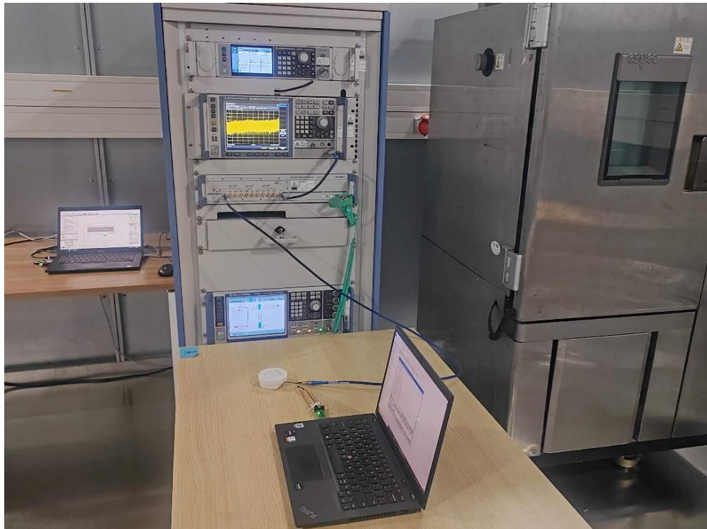
Photograph 1: Set-up photo for RF Conducted Test
