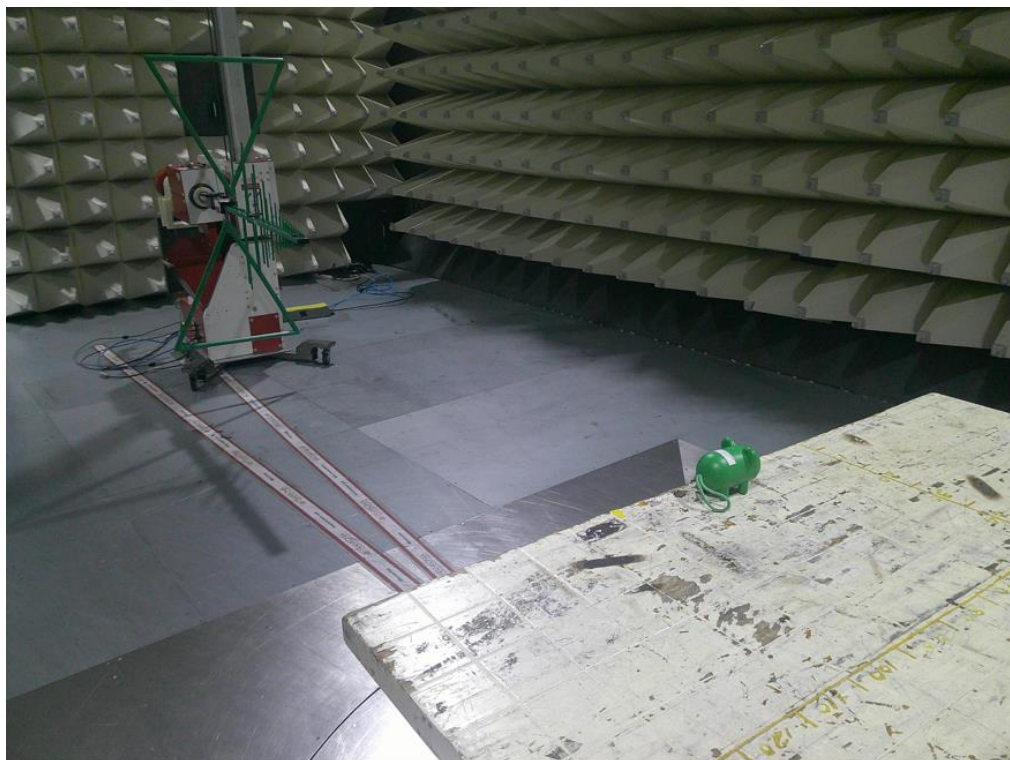
Photograph 3: Set-up photo for Radiated Emission, 30MHz - 1GHz
