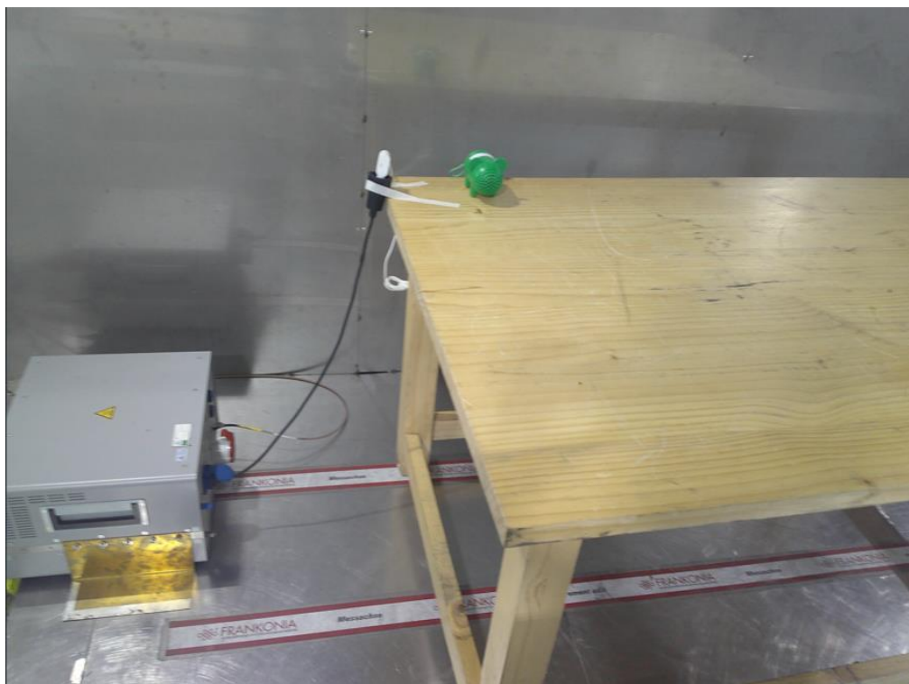
Photograph 2: Set-up photo for Conducted Emission
