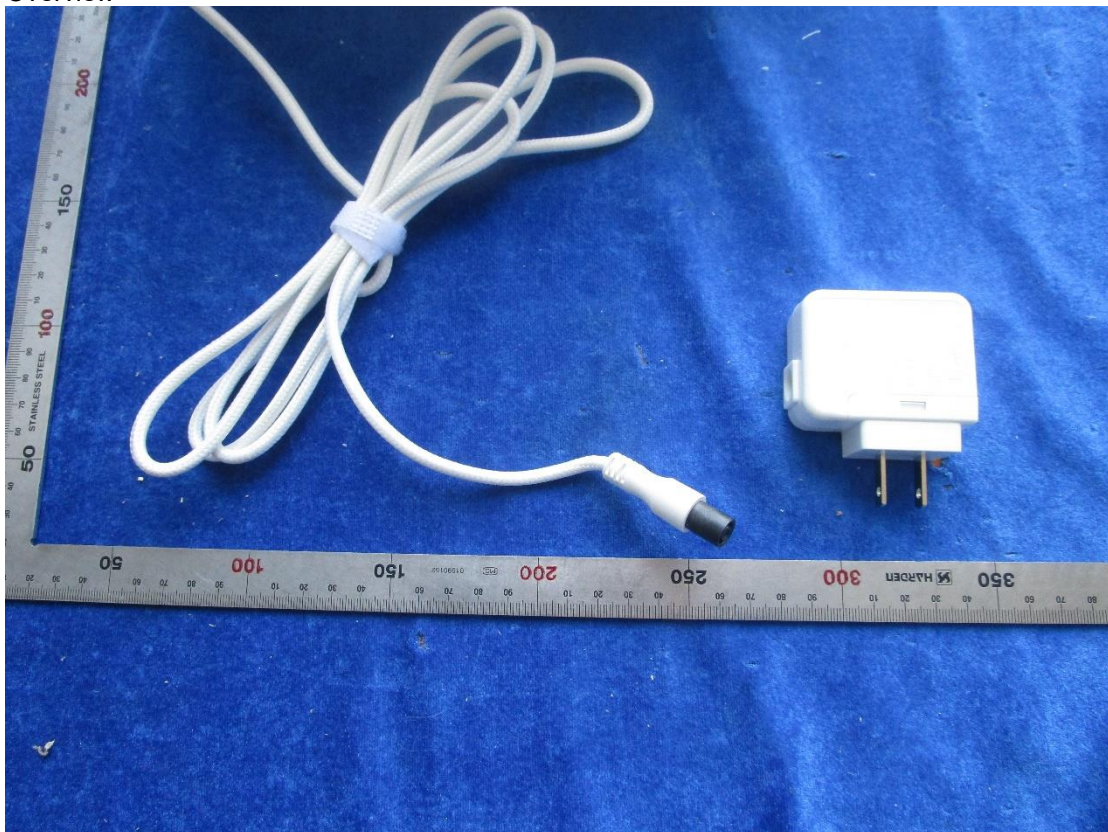
LED driver and DC connector
