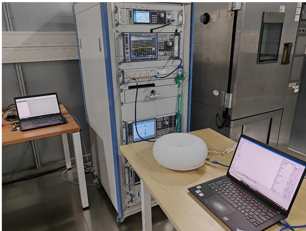
Photograph 1: Set-up photo for RF Conducted Test
