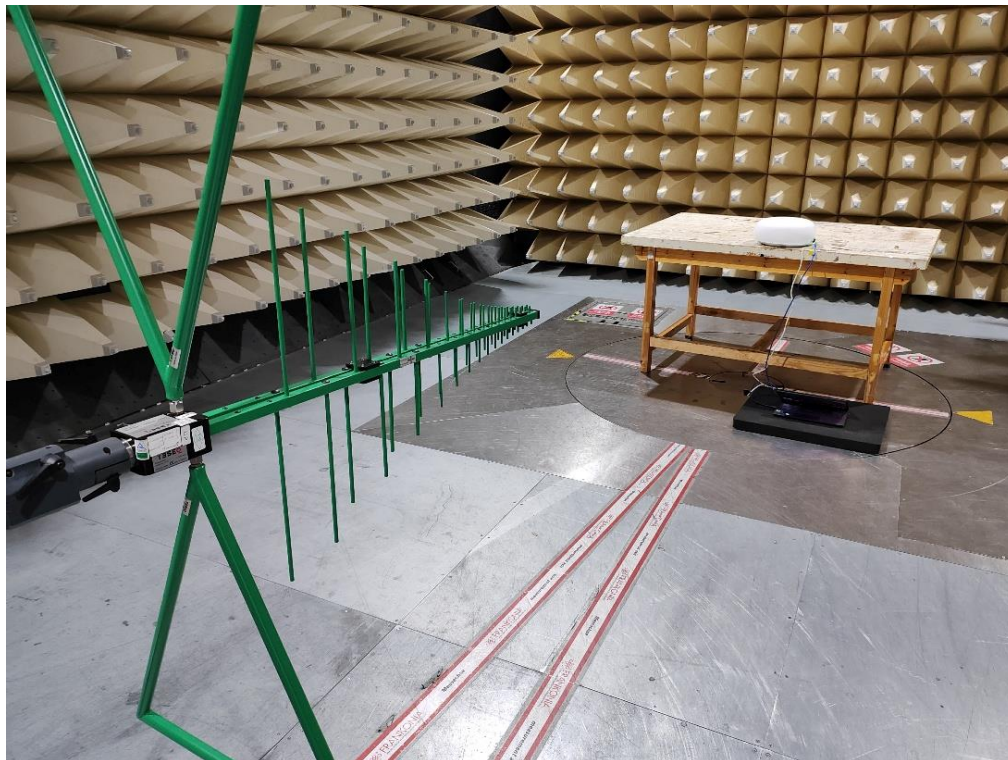
Photograph 3: Set-up photo for Radiated Emission, 30MHz - 1GHz
