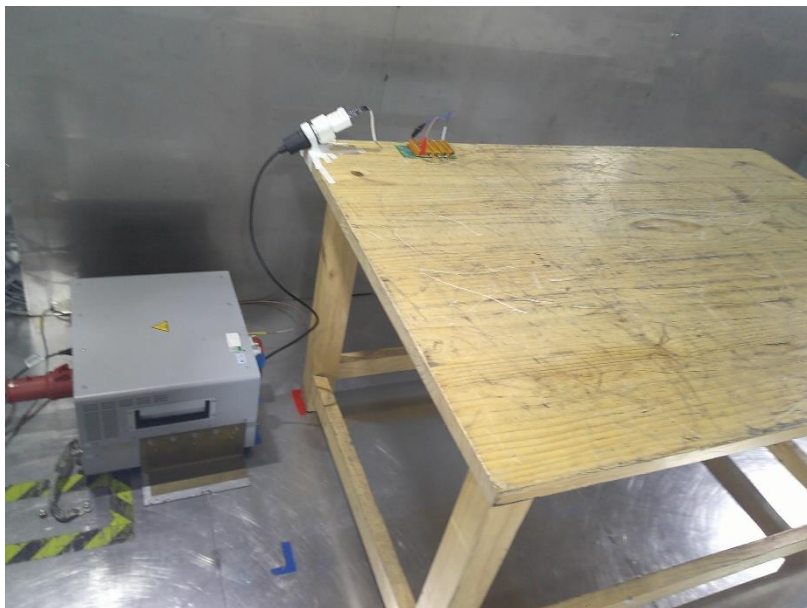
Photograph 2: Set-up for measurement of conducted emission
